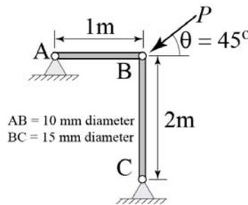
Q.21 The plane frame shown is analyzed by neglecting axial and shear deformations. The horizontal displacement of **joint B** is
